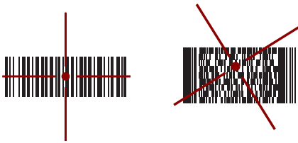
Figure 3-4 Imager Aiming Pattern: Bar Code Centered
